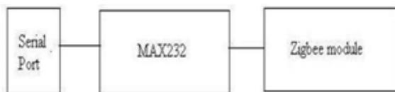
Transmitter Section mainly consists of serial port interfaced to Zigbee Module via MAX232. Module of XBEE Series2 of Digi Inc. [4] has been used. The Xbee radios are programmed using X-CTU software in API mode with the desired baud rate. Screenshots of X-CTU are shown in Net based GUI application is developed on PC which enables the user to display message.
