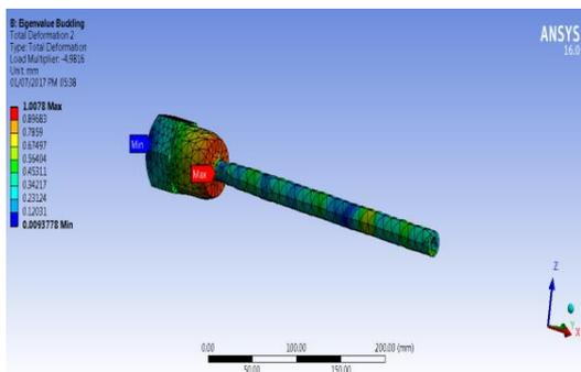
Figur.14. Buckling Mode Shape for optimized Tie Rod
