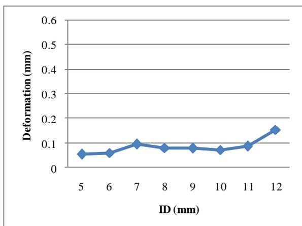
**Figure.18. FE deformation results for different inner diameters of tie rod**
