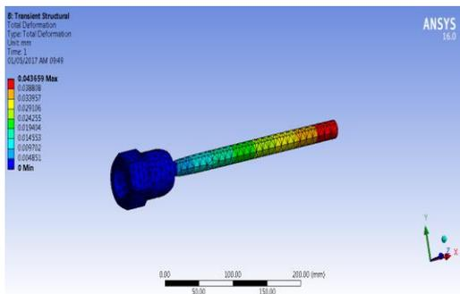
Figure.13. Deformation results
