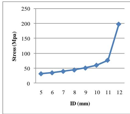
**Figure.19. FE stress results for different inner diameters of tie rod**
