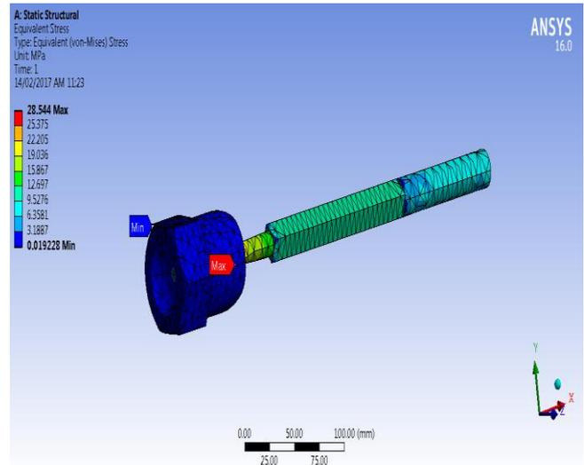
Figure.6. Result for Von-mises stresses for Deformation
