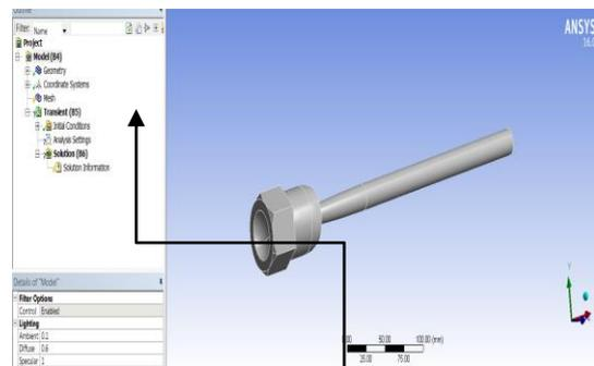
**Figure.11. Model opened in ANSYS workbench for dynamic analysis**
