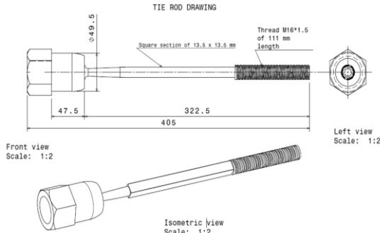
Figure.3. Tie rod drawing
