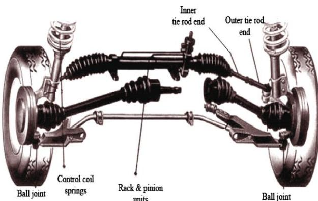
Figure.1. McPherson suspension with rack and pinion.
