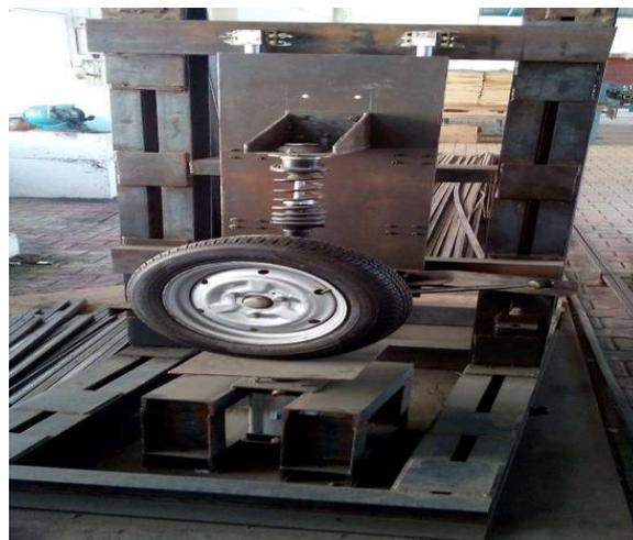
Figure.15. Special designed test rig for testing of Tie Rod
