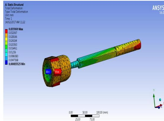
Figure. 5. Result for Deformation
