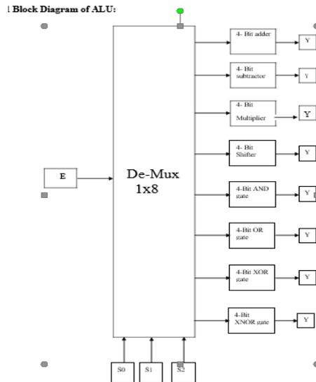
Figure.7. block diagram of ALU
