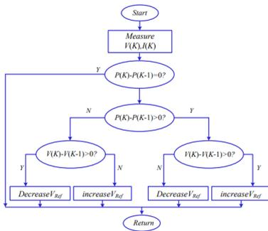
Figure. 3. Flowchart of the P&O algorithm.
