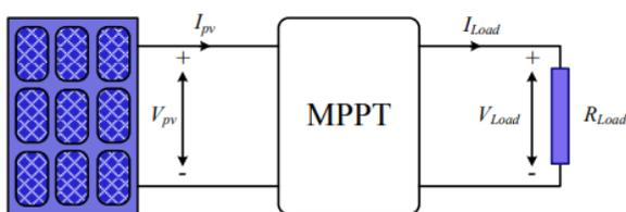
**Figure.1. MPPT Tracking Using Converter**
