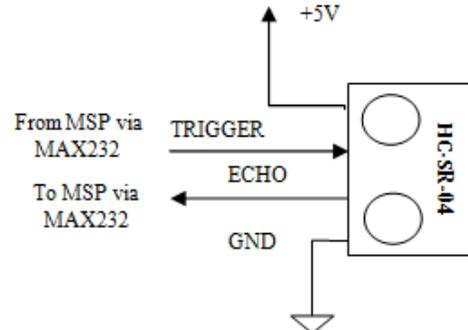
Figure 4. U/S Module Connectors
