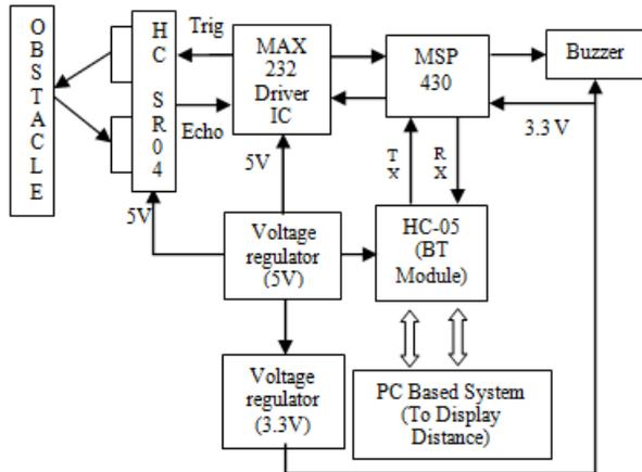
Figure 2. System Configuration
