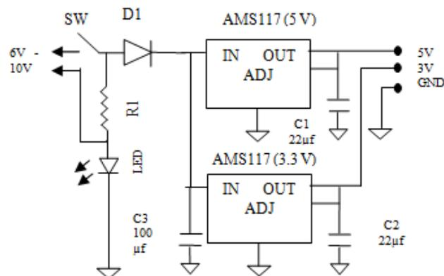
Figure 3. Voltage Distribution Circuit [10]
