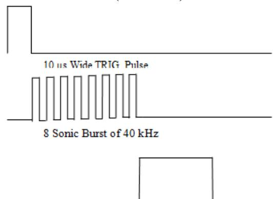
**Figure.1. Hcsr-04 Timing Diagram [9]**
