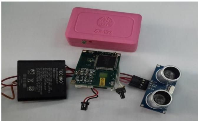
Figure.10. Working Model Of Vision Based System
