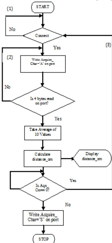
Figure .9. Flowchart of Gui Program
