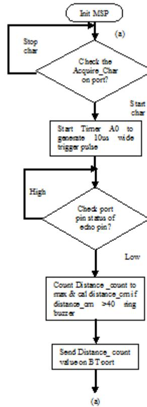
Figure.7. Flowchart of Microcontroller Program
