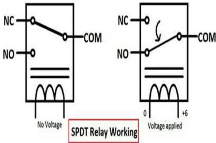
**Figure. 8. The switching unit, SPDT in no voltage and applied voltage.**
