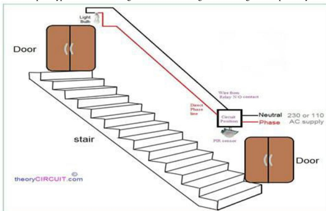
Figure.2. Prototype of sensor based human detector for lighting purpose
