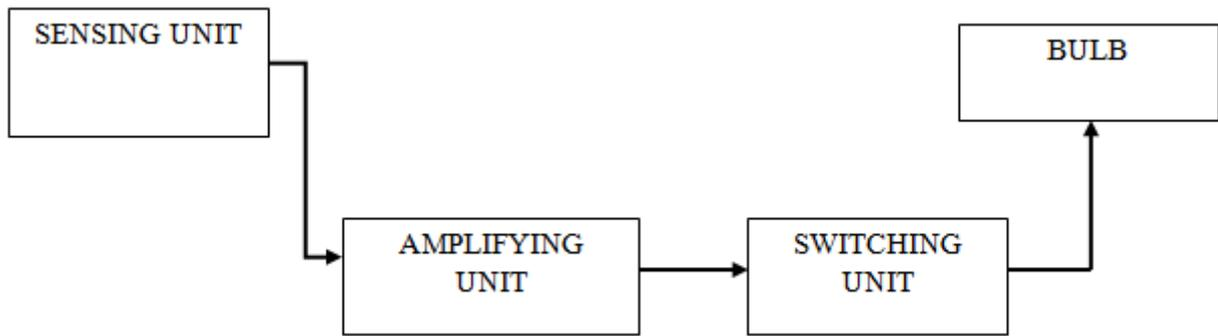
**Figure.3. Block Diagram of sensor based human detector for lighting purposes**
