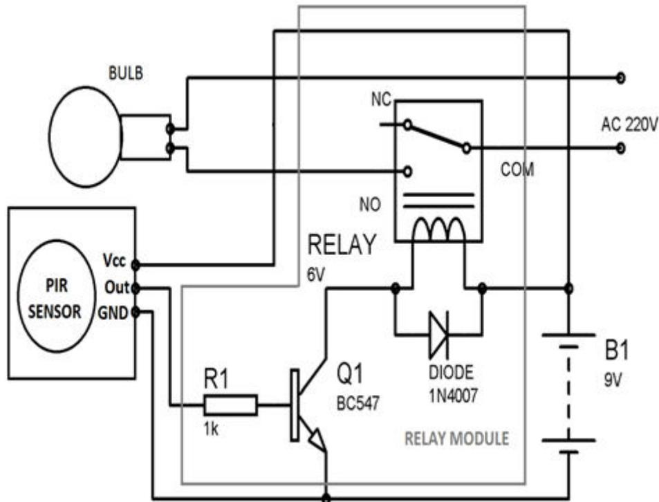
**Figure.4. Circuit layout of the sensor based human detector for lighting purpose on the stair case.**
