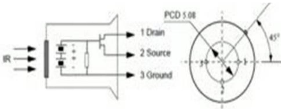
Figure.5. Internal view of Passive Infrared Sensor
