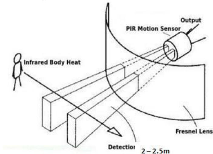
Figure.6. External view of Passive Infrared Sensor
