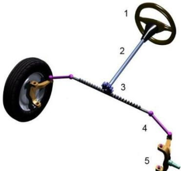
**Figure. 1. Rack and pinion steering mechanism**
