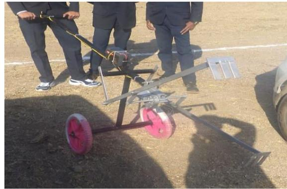
Figure.3. Battery Operated Weeder
