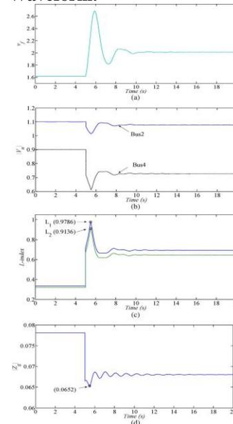
(a) Generator field voltage. (b) Voltage magnitude at buses 2 and 4. (c) L-indices at bus 4. (d) Generator internal equivalent impedance.
