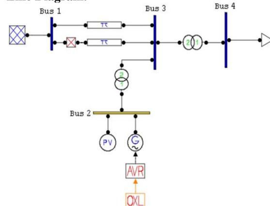
In this project, a generator equivalent model (GEM) is proposed for voltage stability analysis. Based on their dynamic models and real-time measurements, generators are modeled by time-varying internal voltages and impedances to capture the dynamic behaviors of generators. Furthermore, the traditional L-index is extended to incorporate GEMs
