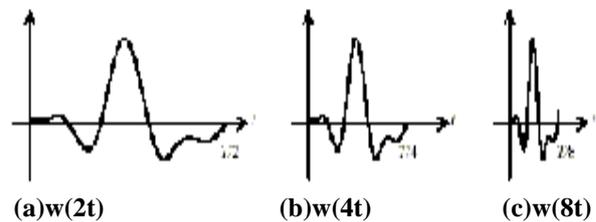
**Figure.4. Scaled wavelets**
