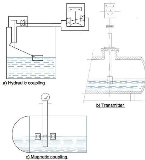
FIGURE 4 MECHANICAL FLOAT METER
