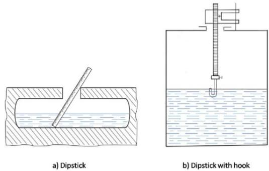
FIGURE 3. SOUNDING LINE METER
