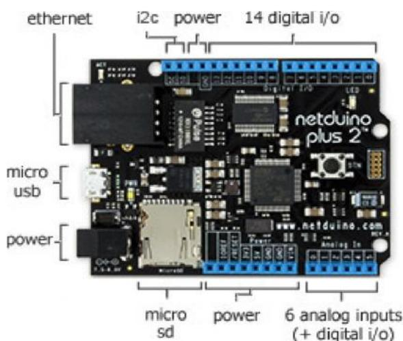
FIGURE 5 NETDUINO PLUS 2 BOARD
