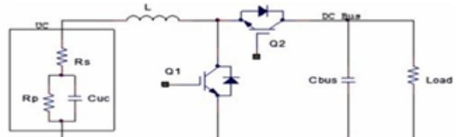
Figure.4. The electrical circuit of ultra-capacitor-bidirectional DC-DC converter topology
