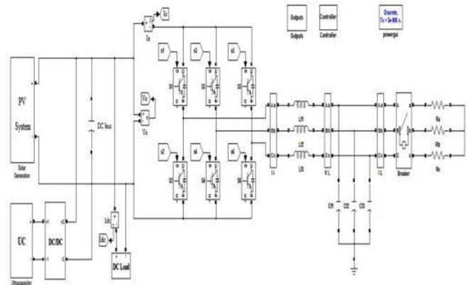
**Figure.5. simulation diagram of the proposed system with ultra- capacitor and PV system**
