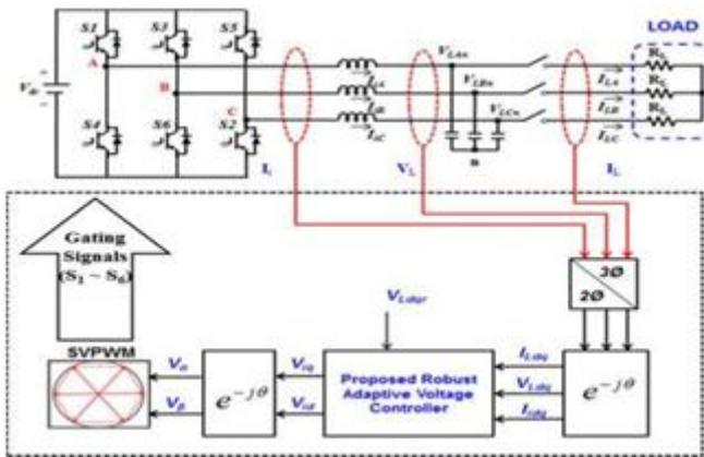
Figure.2. Schematic diagram of a three-phase dc to ac inverte
