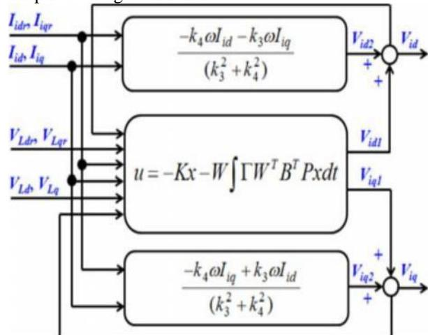
Figure.3. Block diagram of the proposed adaptive voltage controller
