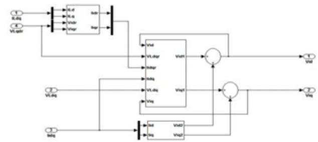
**Figure.7.adaptive voltage controller**
