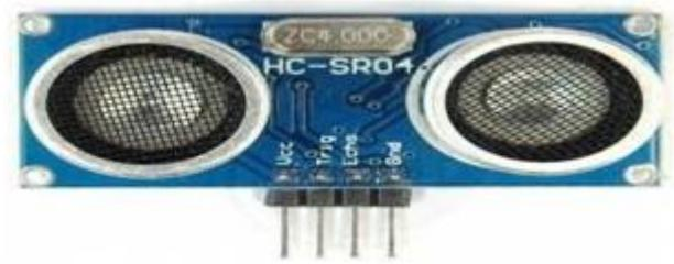
Figure.4. HC-SR04 ultrasonic distance sensor used in the system
