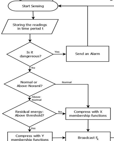
Figure.2. Adaptive Encoding Algorithm 3
