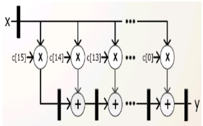
Figure.5. Architecture of FIR filters.
