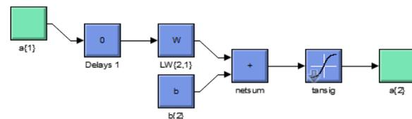
Fig. 4: Layer 2 of Feed Forward Neural network model
