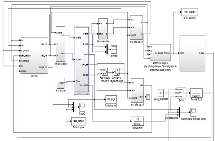
Fig.1: Proposed simulation model for speed estimation
