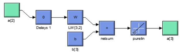
Fig. 5: Layer 3 of Feed Forward Neural network model
