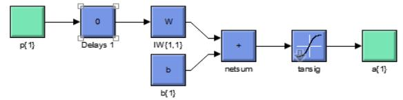
Fig. 3: Layer 1 of Feed Forward Neural network model
