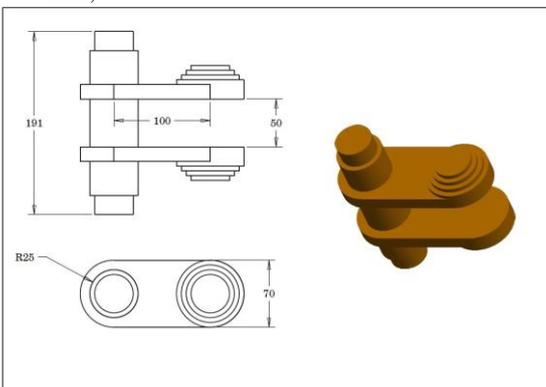
Figure.4. Design of Vibratory Shaft
