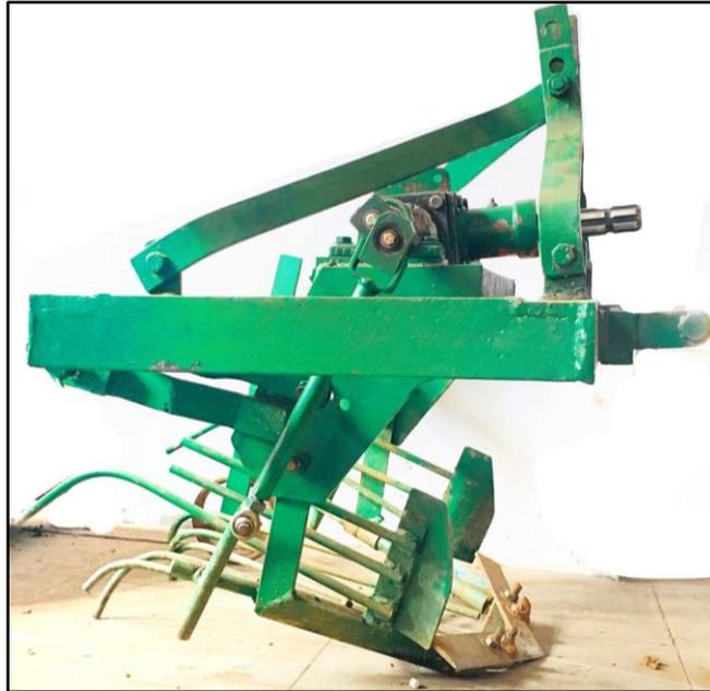
**Figure.4. Side view of Mini Tractor operated Coleus diggerR**
