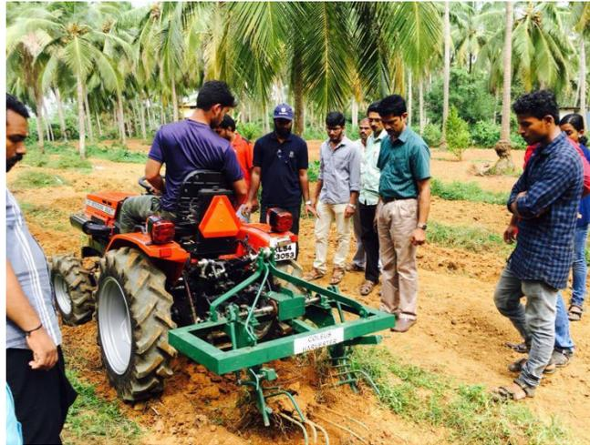
Figure .1. Mini-tractor driven coleus digger
