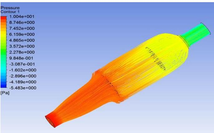
**Figure.7. CFD of corrugated shaped substrate within the converter**
