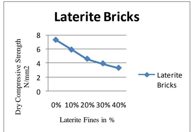
**Figure.1. Variations of Compressive strength for Dry bricks with varying laterite fines**
