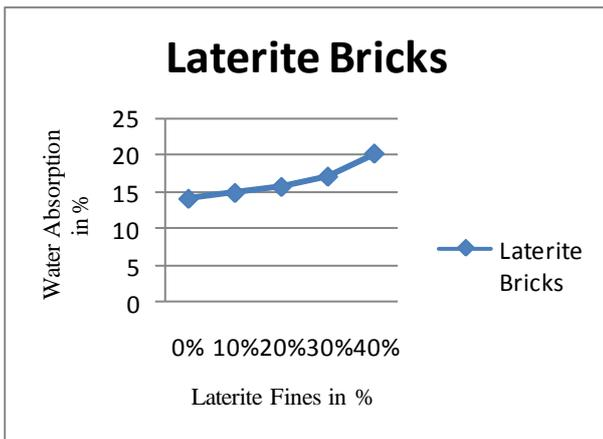
**Figure.3. variation of water absorption characteristics of bricks with varying laterite fines**
