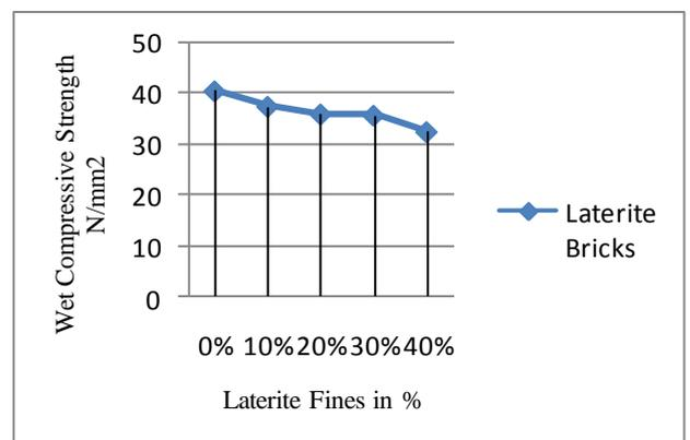
**Figure.2. Variation of Compressive strength for wet brick with varying Laterite fines**
