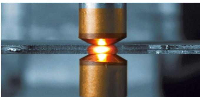
Figure 3.8 Resistance Welding
