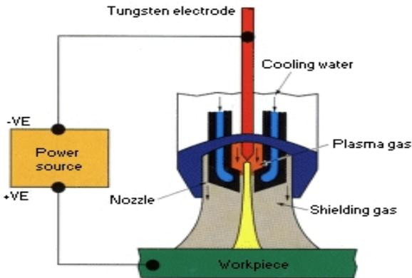
Figure 3.7 Plasma Arc Welding
