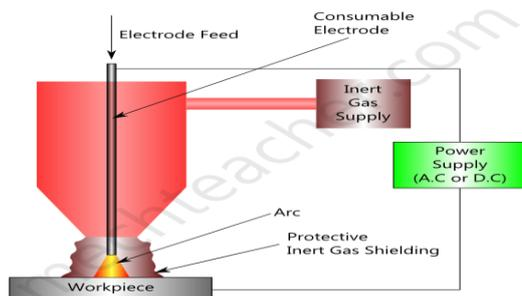
Figure 3.4 Metal Inert Gas Welding
