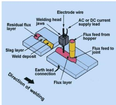
Figure 3.3 Submerged Arc Welding
