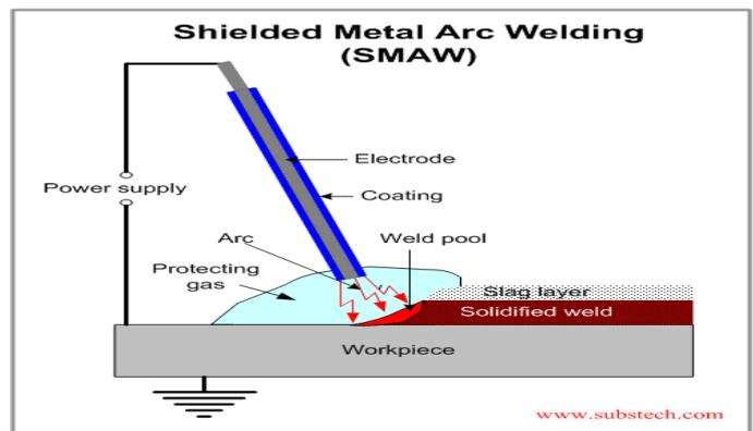
Figure 3.2 Shielded Arc Welding
