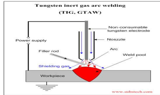
Figure 3.5 Tungsten Inert Gas Arc Welding
