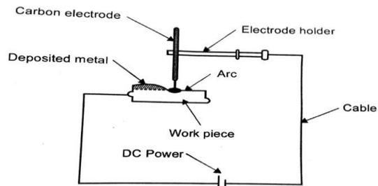
Figure 3.1 Carbon Arc Welding
