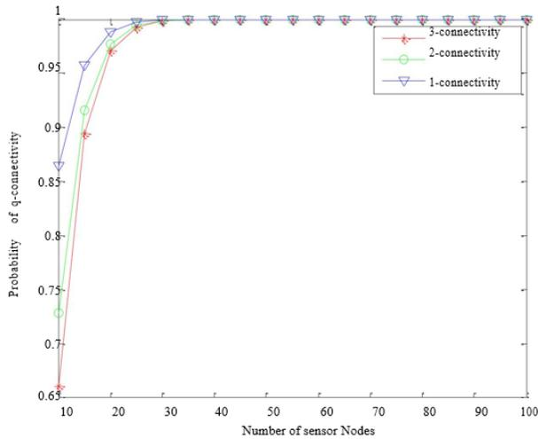
**Figure.9. Probability of  $q$ -connectivity versus number of sensor nodes ( $A=1000 \text{ m}^2$ )**
