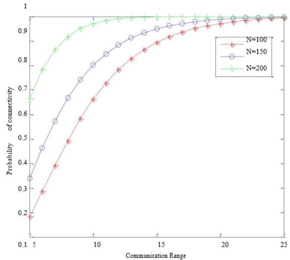
**Figure.11. Probability of Connectivity versus communication range ( $A=1000 \text{ m}^2$ )**
