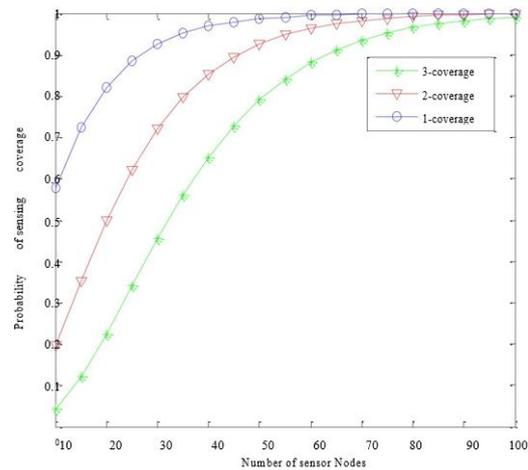
**Figure.8. Coverage probability versus sensor nodes at standard deviation = 2 (A=3000 m<sup>2</sup>)**
