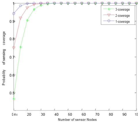
**Figure.4. Coverage probability versus sensor nodes at standard deviation = 2 (A=1000 m<sup>2</sup>)**
