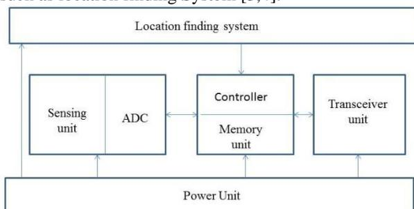
**Figure.1. Hardware Architecture of a Sensor Node**
