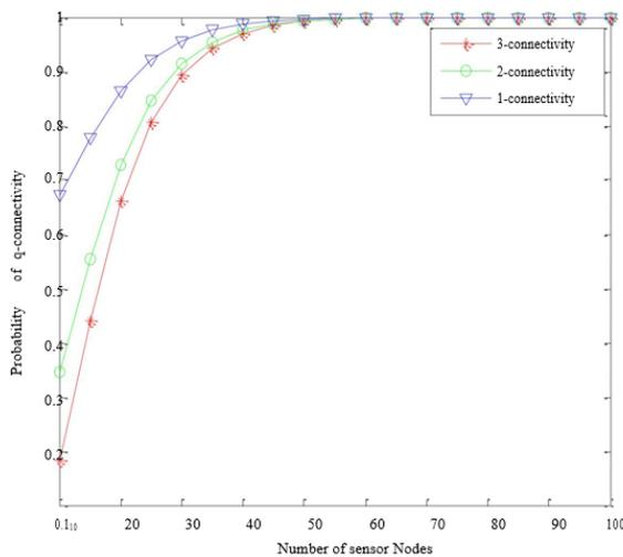
**Figure.10. Probability of  $q$ -connectivity versus number of sensor nodes ( $A=2000 \text{ m}^2$ )**
