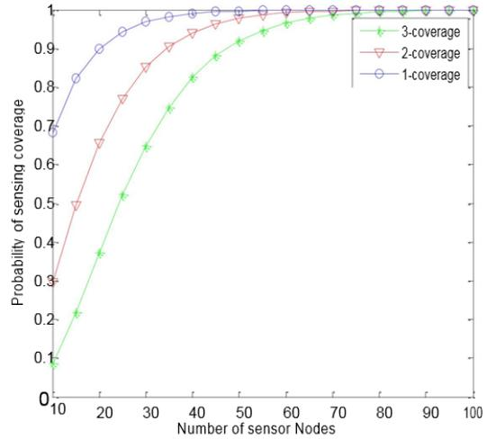
**Figure.7. Coverage probability versus sensor nodes at standard deviation = 4 (A=2000 m<sup>2</sup>)**
