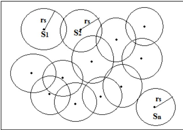
**Figure.2. Coverage in Wireless Sensor Networks**
