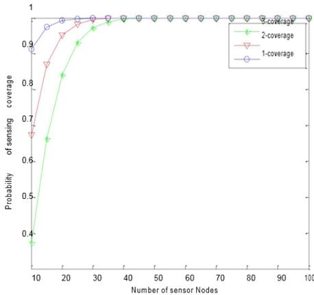
**Figure.5. Coverage probability versus sensor nodes at standard deviation = 4 (A=1000 m<sup>2</sup>)**
