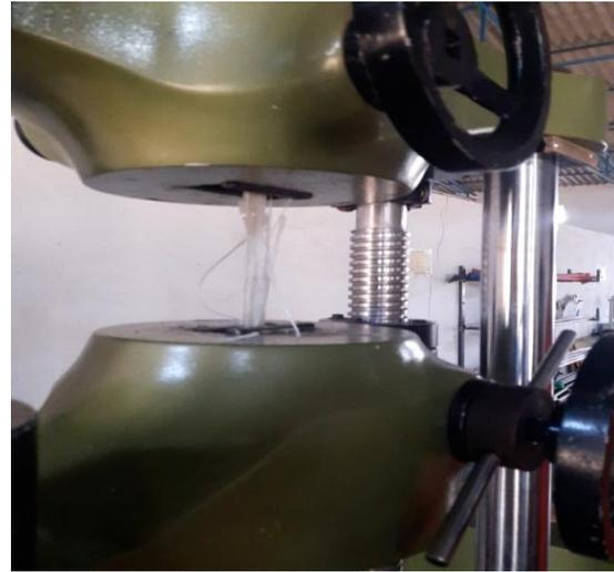
Figure .14. Fracture occurs on UTM
