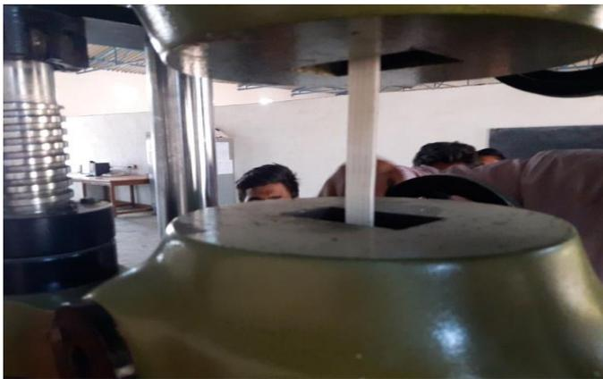
Figure.13.Specimen Placed in UTM for tensile test
