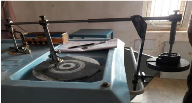
Figure.12.Pin-on Disc Setup for Wear Test
