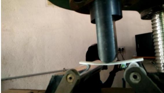
**Figure.17. Specimen Placed in UTM for Flexural test**
