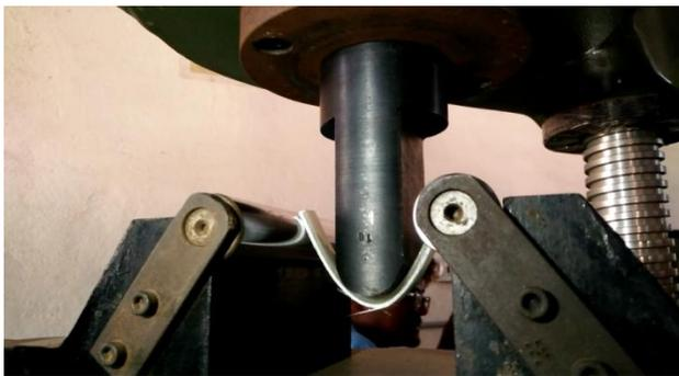
**Figure.18. Bending Occurs on UTM**
