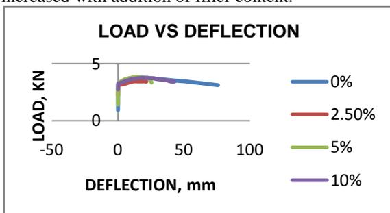
**Figure.19. Load vs Deflection Graph for Flexural Test**
