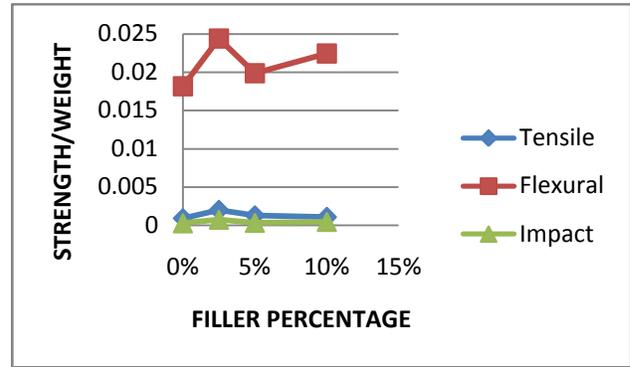
**Figure.23. Weight to Strength Ratio Graph**
