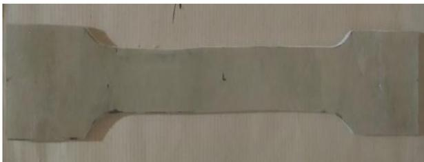
Figure.8. Tensile test Specimen
