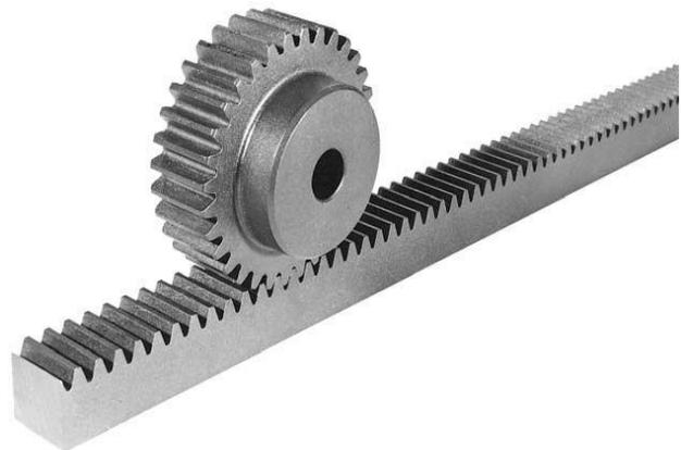
The rack carries the full load of the actuator directly and so the driving pinion is usually small, So that the gear ratio reduces the torque required. This force, thus torque, may still be substantial and so it is common for there to be a reduction gear immediately before this by either a gear or worm gear reduction. Rack gears have a higher ratio, thus require a greater driving torque, than screw actuators.
