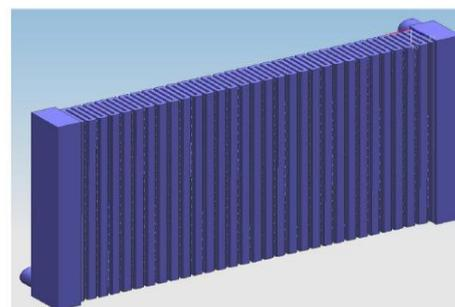
**Figure.2. carbon foam radiator concept**
