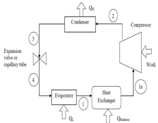
**Figure.1. Basic Refrigeration Cycle with Additional Heat Exchanger**
