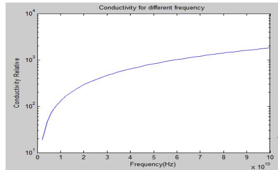
**Figure 4**Conductivity in funfunction to the frequency.
