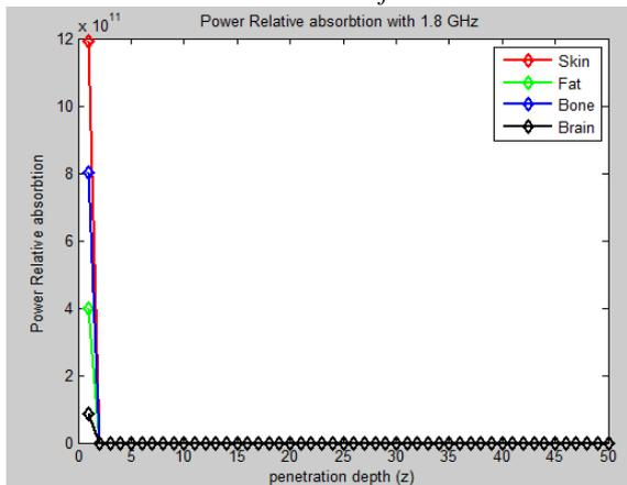
**Figure10.** Power absorptive in function to depth  $z$  for  $f=1.8\text{GHz}$ .
