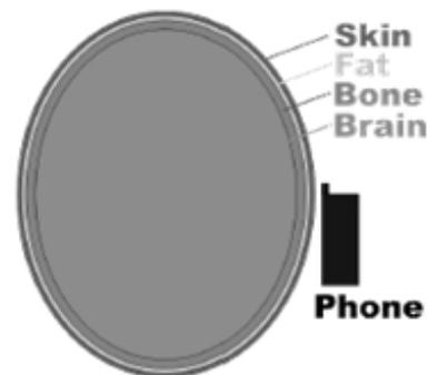
**Figure 2 Simple models of the human head (Reference 6)**
