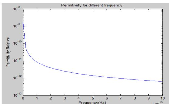
**Figure 3.** Relative permittivity in function to the frequency
