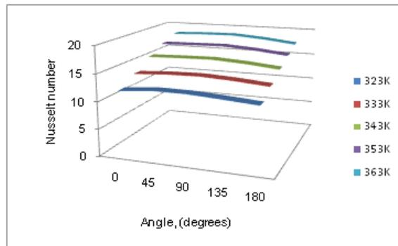
Figure 8. Graph showing the nusselt number along a vertical line for different orientations and base temperatures.
