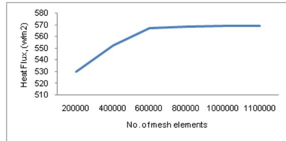
Figure 3. Graph showing the variation of heat flux and the number of mesh elements
