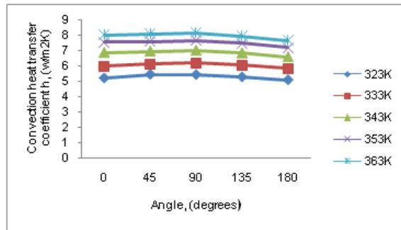
Figure 7. Graph showing the convection heat Transfer coefficient on the vertical line For different orientations and base temperatures
