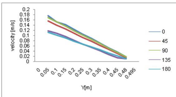
Figure 6. Graph showing the velocity along a vertical line for the different angles
