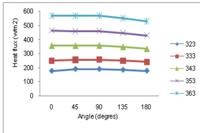
Figure 9. graph showing the heat flux along a vertical line for the different orientations and base temperatures.
