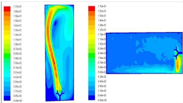
Figure 4. Velocity Contours Of Orientation  $0^\circ$  And  $90^\circ$  For 333k Base Temperature
