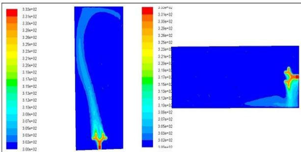
Figure 5. Temperature Contours Of Orientation  $0^\circ$  And  $90^\circ$  For 333k Base Temperature
