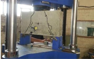
Figure.1. Test Setup of UTM with Roller Base for Shear
