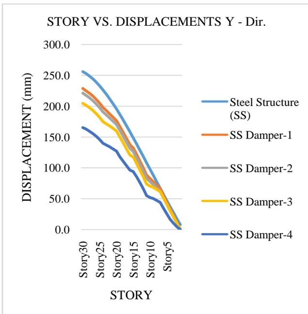
Figure.0.3. Story vs Displacements – Y Dir.
