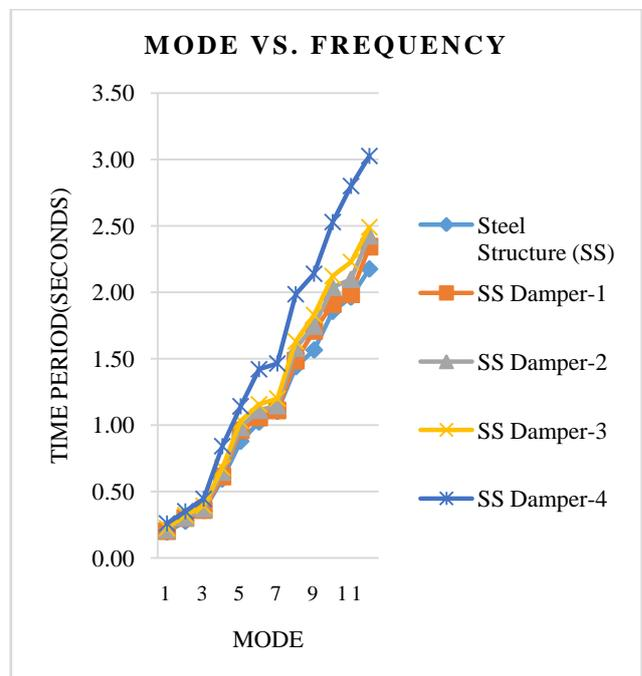
Figure.0.1. Mode vs. Frequency
