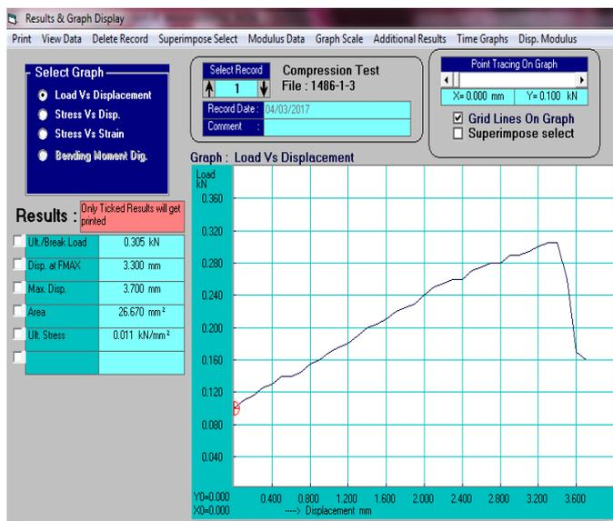
Figure. 3. Load vs Displacement Graph for Jute fiber
