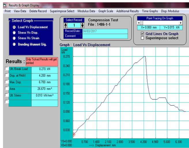
Figure .2. Load vs Displacement Graph for Glass fiber
