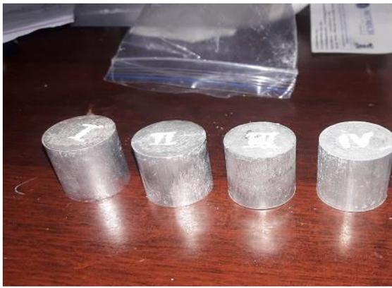
Figure.3.2. Compacted composite samples
