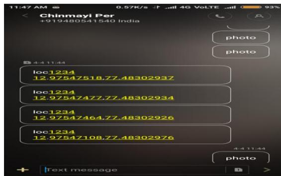
Figure.9. If the guardian wants to track the location of victim then he depresses the track button in his app, so that the location of victim is obtained to guardian in terms of latitude and longitude points.
