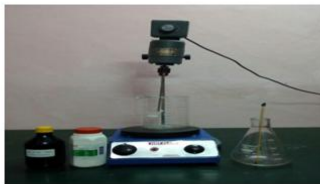
Figure.2. Photographic view of biodiesel preparation plant (Transesterification process)
