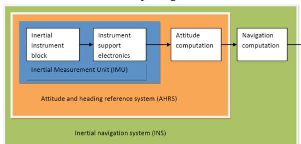
**Figure.2. Building Blocks of the strapdown INS System**
